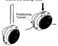
Pull the line and make sure the line is against the hub and extended full through the positioning tunder.
